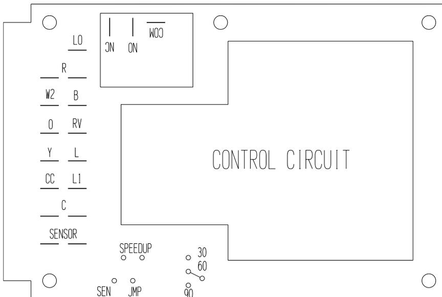
There is a cycle speed up jumper on the control. This can be used to reduce the time between defrost cycle operation without waiting for time to elapse.
