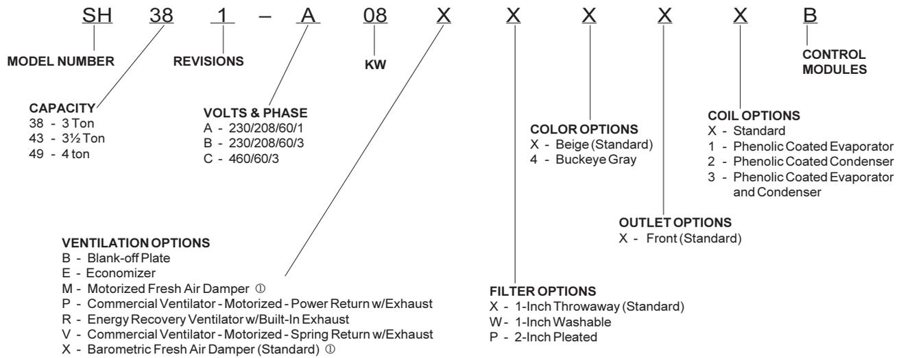
① Vent options are without exhaust capability. May require separate field supplied barometric relief in building.
