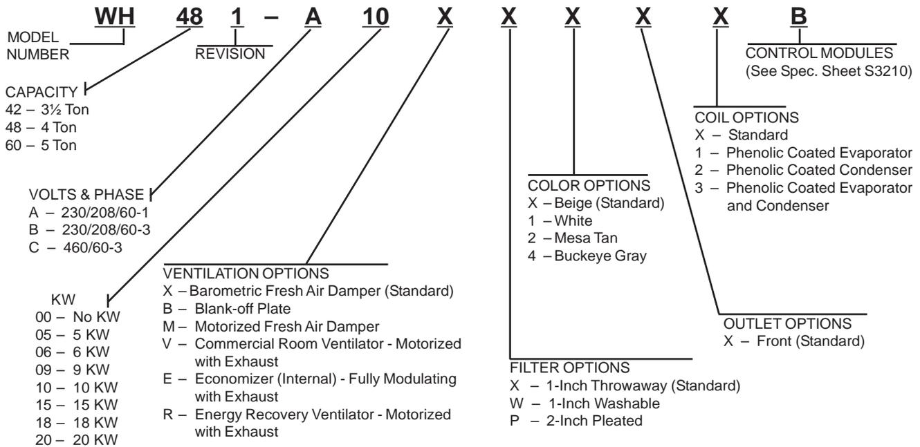
NOTE: For 0KW and circuit breakers (230/208V) or pull disconnects (460V) applications, insert 0Z in the KW field of model number.
