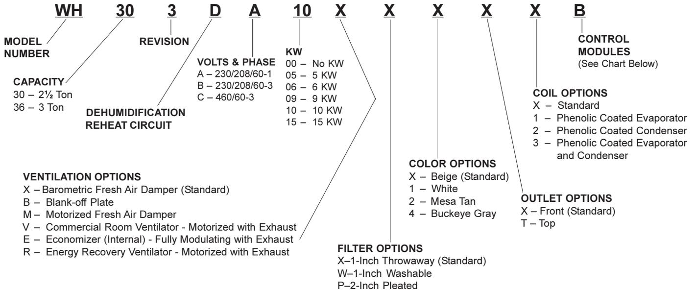
NOTE: For 0 KW and circuit breakers (230/208 V) or pull disconnects (460 V) applications, insert 0Z in the KW field of model number.
