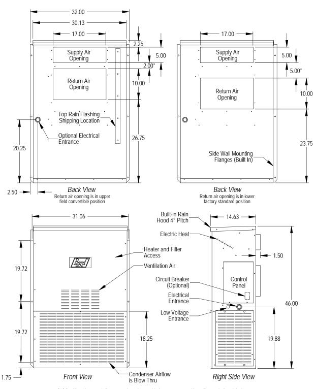
(\*) Position of return air flanges are interchangeable between two positions. Factory built at 5 inches. Note: Maintain a minimum of 20 inches clearance on right side to allow access to control panel and allow proper airflow to outdoor condenser coil. Allow 15 inches on left side.
