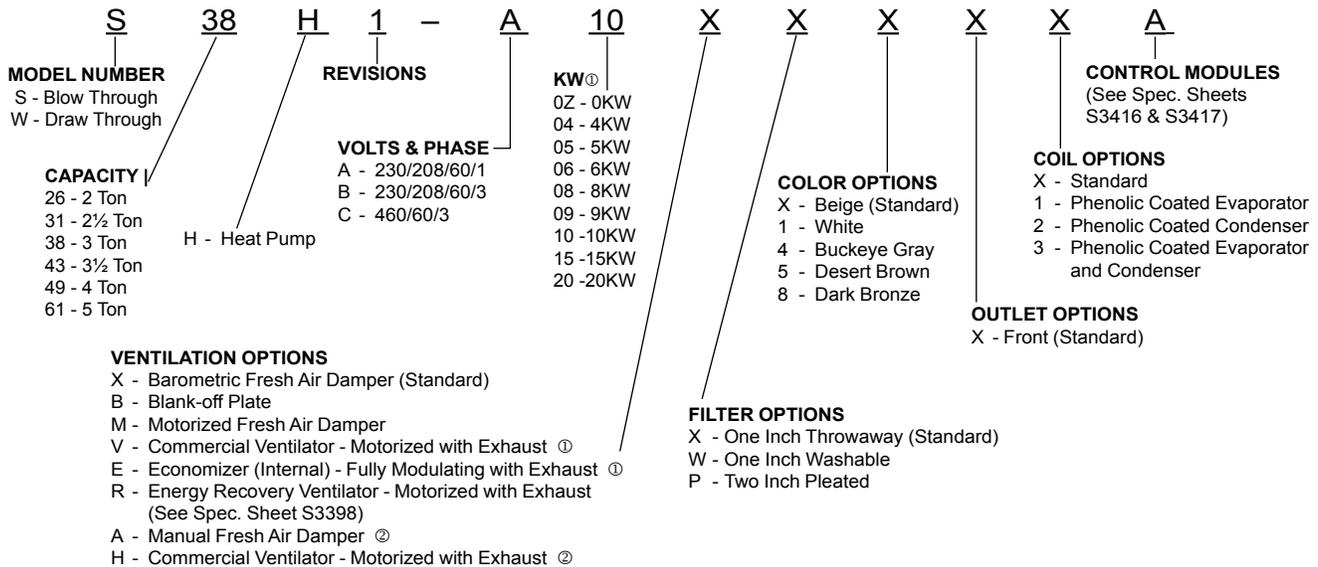
**NOTE:** Vent options X, B and M are without exhaust capability. May require separate field supplied barometric relief in building.
