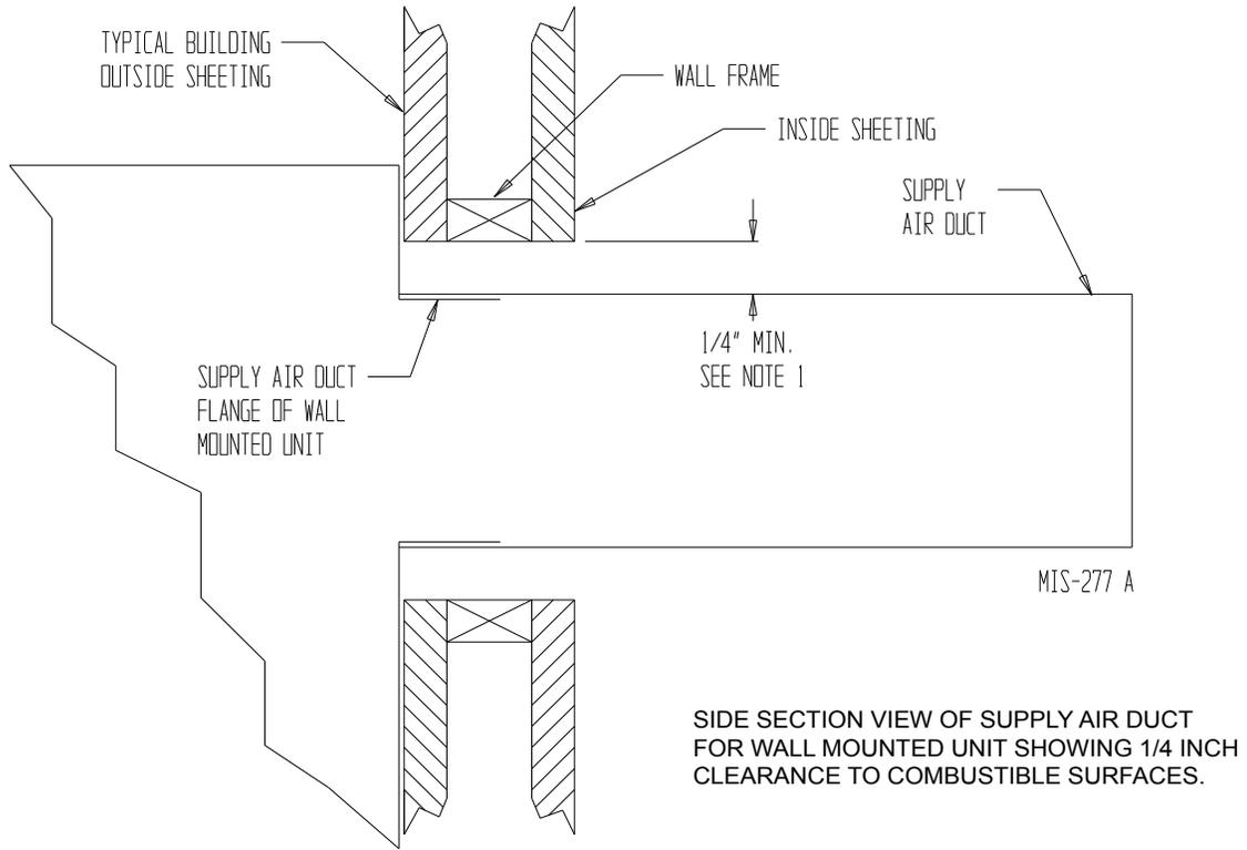
SIDE SECTION VIEW OF SUPPLY AIR DUCT FOR WALL MOUNTED UNIT SHOWING 1/4 INCH CLEARANCE TO COMBUSTIBLE SURFACES.
