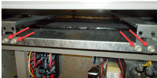
FIGURE 6 Remove Four Screws
