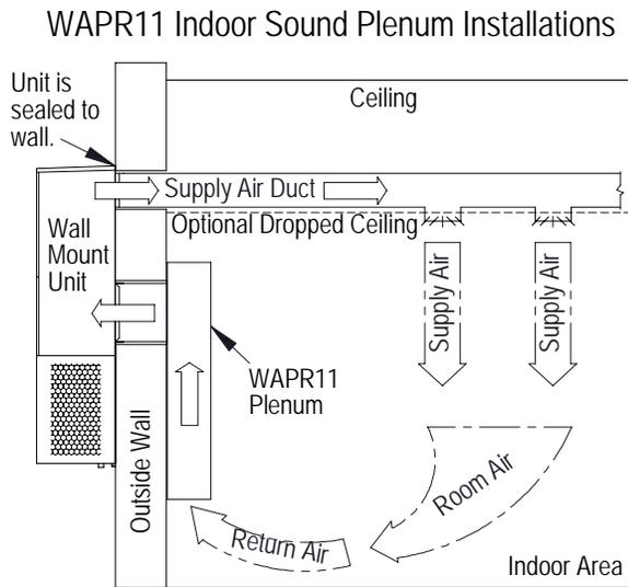
Indoor sound plenums are installed inside the room over the unit return air opening. Plenum use can provide sound isolation and indoor area sound reduction. The WAPR11 sound plenum provides a single solution for all unit tonnage sizes. The WAPR11 may be installed horizontally or vertically in the room. Unit duct static requirements cannot be exceeded when using a sound plenum. Follow all instructions provided with the sound plenum when installing the product.
