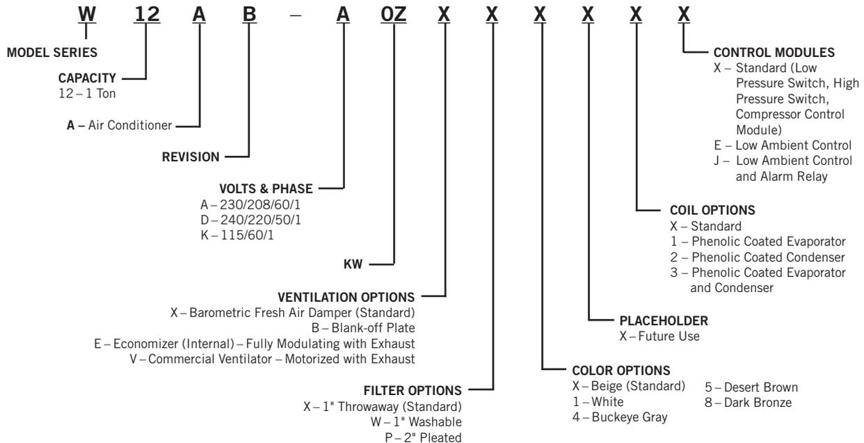
**NOTE:** Vent options X and B are without exhaust capability. May require separate field-supplied barometric relief in building.
