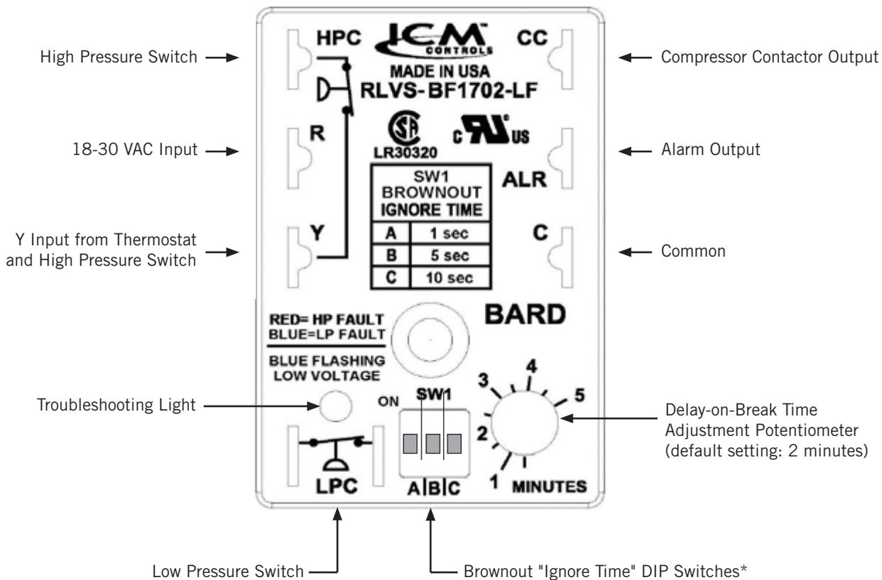
\* Turn on only one switch for that specific "Ignore Time" setting. 10 seconds is the maximum brownout "Ignore Time". If all switches are "off", the control is in "do not ignore".
