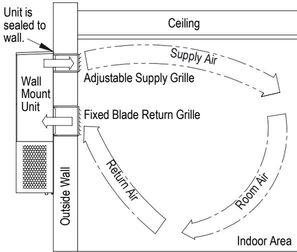
Non-ducted installations supply conditioned air into indoor room areas without extensive duct work. The supply airstream is directed by adjusting the 4-way supply grille to reach areas being conditioned. The supply air mixes with the room air and cools or heats occupants and/or equipment in the area. Unconditioned room air is returned to the unit through the return grille. Avoid supply air leaving supply grille and re-entering the unit return grille without mixing with room air.
