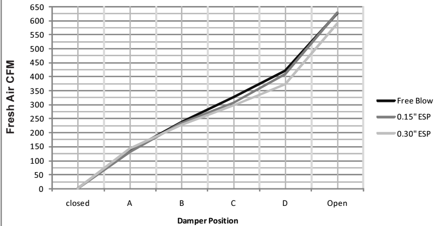
W42-60G CRV Airflow Versus Position - Low Speed
