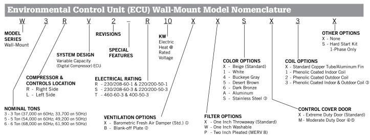
① Vent option X does not have exhaust capability. May require separate field supplied barometric relief in building.
