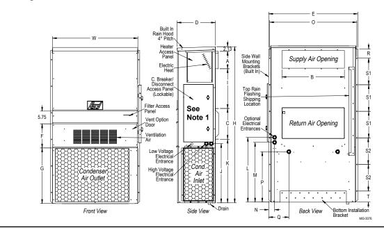
**Note 1:** Extreme Duty control panel door is shown and is standard. For optional flush Moderate Duty Control Panel Cover, order Control Cover option "M". See Nomenclature on Page 8.
