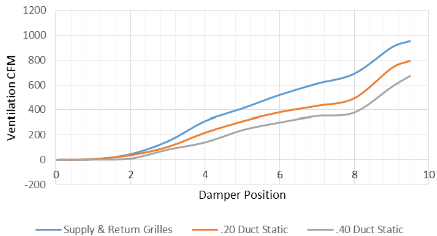
W42 and W48 Ventilation Delivery
