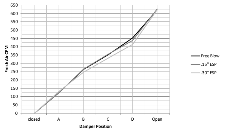
W60G4 CRV Airflow Versus Position - Low Speed
